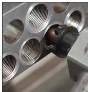
Safely re-machine gasket surfaces in seconds.
