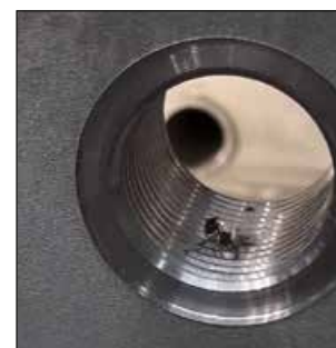
All types of water box materials can be machined with the carbide inserts of the MiniMill 300 GFF.
